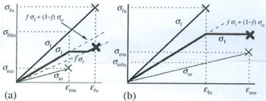
3. A cross-ply laminate (E-glass/epoxy) is loaded under tension to final fracture. Explain how the failure proceeds and give reasons why so. (10p)
